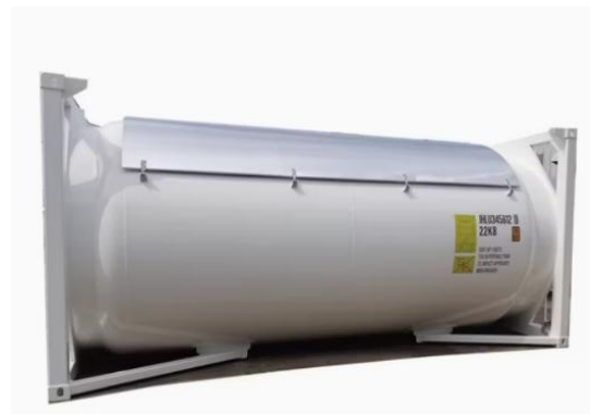
Figure 5 - ISO Container fitted with sun shield (courtesy Fogas)
