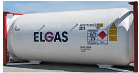
Figure 7 - LPG ISO container hazard labels (Courtesy of Elgas Australia)
