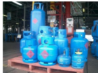
Typical sizes of steel LPG cylinders used in the residential, commercial and industrial sectors
