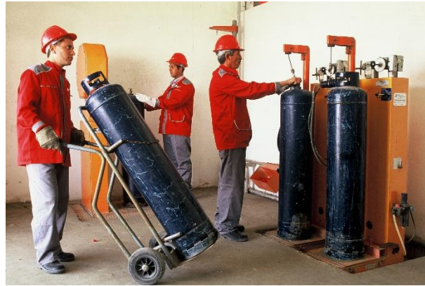
Barrows with retaining chains are useful when moving 45 kg industrial cylinders over short distances
