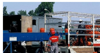
Portable conveyor being used to load/unload cylinders from vehicle
