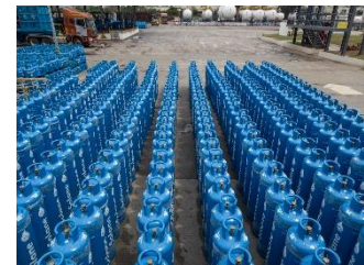
Leave access rows when storing LPG cylinders
