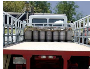
Rows of cylinders on vehicle separated by wooden sheet
