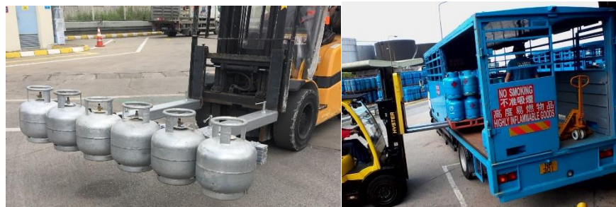
The use of forklift trucks to handle cylinders not only reduces the risk of impact damage it reduces the risk of personnel injuries
