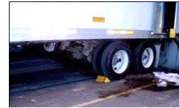
Prevent wheels moving with chocks
