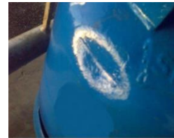
This damaged cylinder should be rejected
