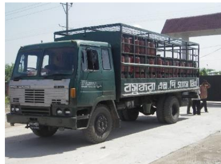
LPG vehicles should securely contain the cylinders during transit and when parked
