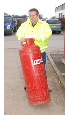
Large cylinders may be rolled on their base although this is to be avoided if alternative options are available
