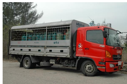
Vehicles should be well ventilated and designed to secure the load
