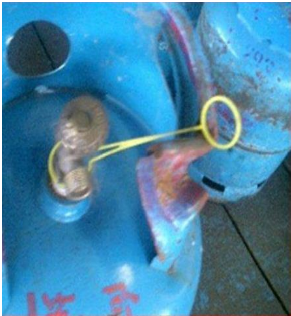
Fig.A.3.4 Example of Collar damage
