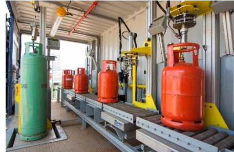
Filling LPG cylinders in a container
