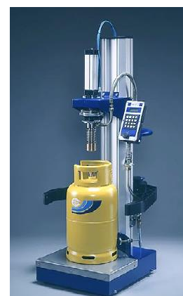
Filling of an industrial cylinder
