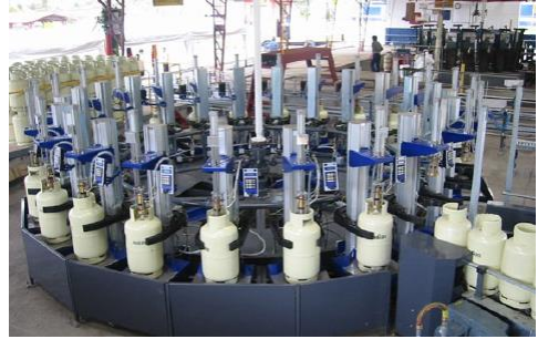
A 24-head carousel in operation
