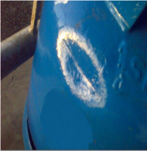
Fig. A.3.1 Examples of dent defects
