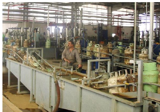
Fully submerged leak detection bath integrated with chain conveyor
