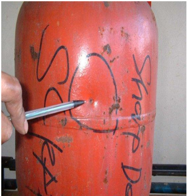
Fig.A.3.5 Example of gouge defect
