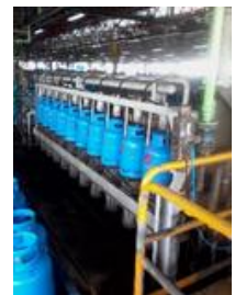
A hydraulic test shown above is normally included in the requalification procedures
