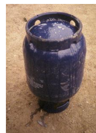
Leaking cylinder identified during post-filling checks
