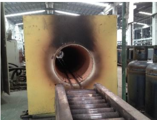
An annealing oven at a cylinder manufacturer
