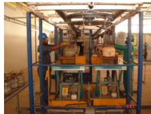
Cylinders loaded in the furnace to be annealed
