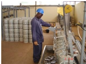
Pressure control and leakage testing
