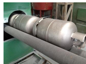
Shot blasting before applying surface finish
