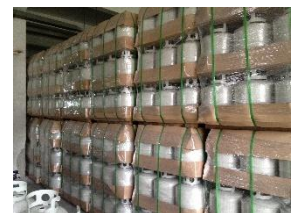
Specifying adequate packing instructions will prevent damage to cylinders during shipping
