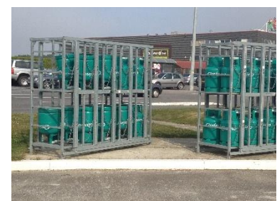
The use of cages at retail sites will increase security and minimise manual handling
