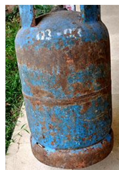
The application of a zinc metallised coating under the final paint finish will prevent this aggressive corrosion. The ventilation holes are small too in this cylinder
