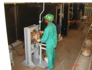
Rectification of the foot ring
