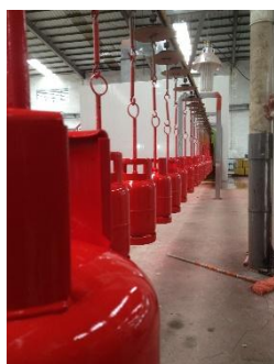
Cylinders receiving top coat of paint
