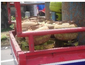
Cylinders with badly damaged foot-rings
