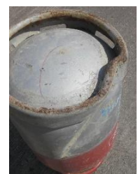
This cylinder suffered severe impact damage in the market making it dangerous and unfit for service
