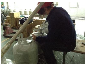
Final internal inspection of cylinder for contamination
