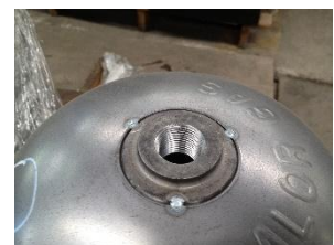
The quality control of the boss and valve threads is a critical item to avoid leakage in service
