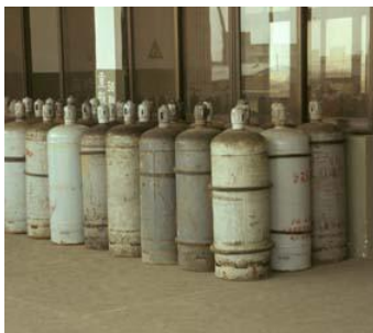
Rubber bands being used on cylinders for protection against abrasion
