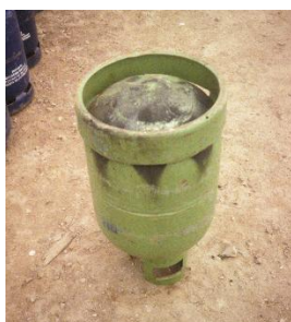
A lighted candle was placed under this cylinder resulting in the paint being burnt exposing the metal
