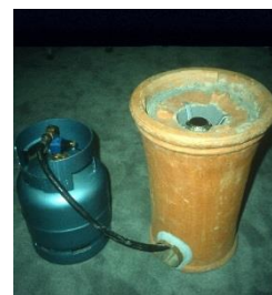
Figure 2.2.2d – Coal briquette burner modified to use LPG (4.5kg cylinder)
